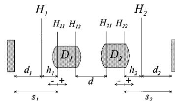
Fig. 8. Plane-plane resonator containing a lens system of thick lenses.
