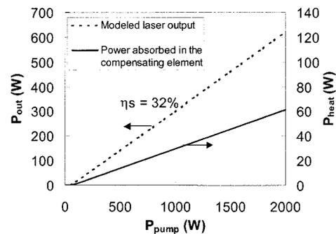
Fig. 2. Performance of the modeled laser and the power absorbed in the compensating element.
