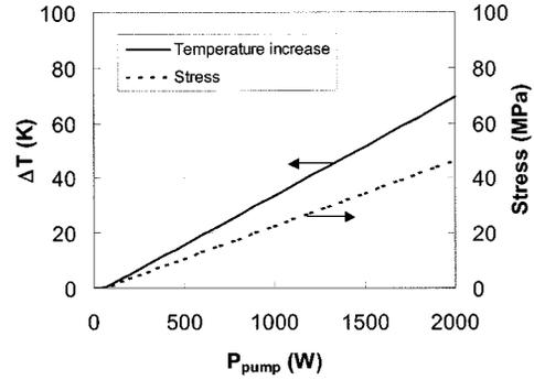
Fig. 4. Calculated temperature increase and maximum tensile stress in the compensating element.
