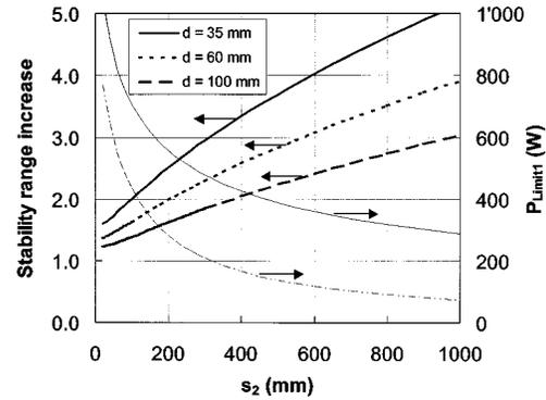
Fig. 6. Increase of the width of the first stability range as a function of  $s_2$  for different  $d$ . The thin lines are the pump power at the first stability limit for  $d = 60$  mm for the “normal” resonator (dashed line) and the compensated system (solid line).
