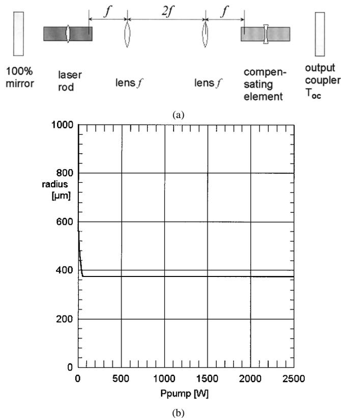
Fig. 7. (a) Imaging resonator arrangement with (b) calculated fundamental mode size in the laser rod.
