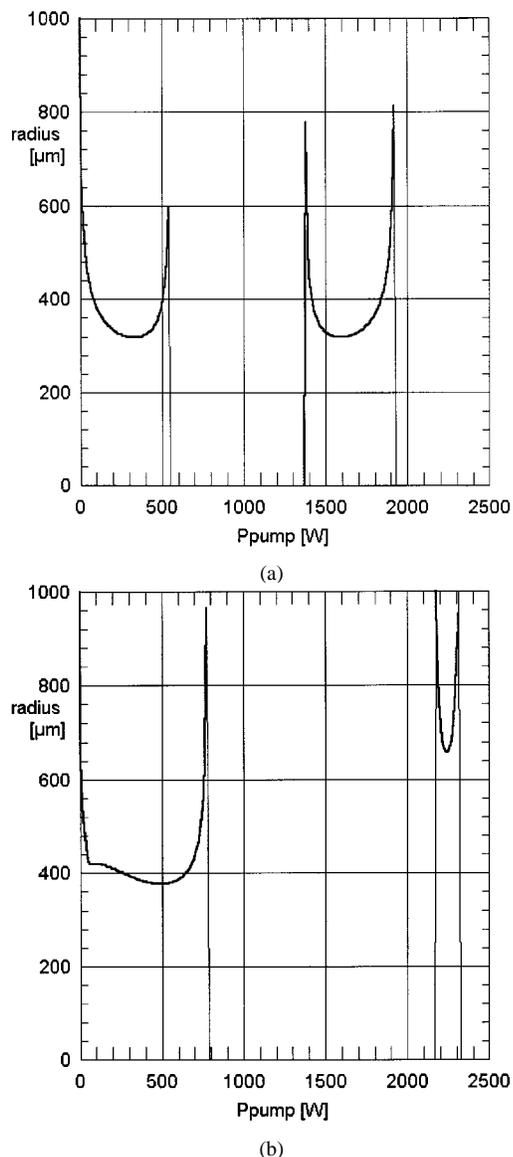
Fig. 5. Stability with increase. (a) Without compensating element,  $\Delta P \approx 550$  W,  $M^2 \approx 20$ . (b) With compensating element,  $\Delta P \approx 800$  W,  $M^2 \approx 12$ .
