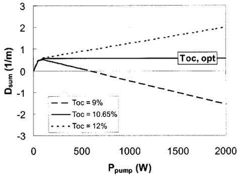
Fig. 3. Sum of the dioptric powers of the two thermal lenses for different output coupler transmissions.
