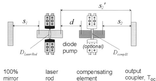
Fig. 1. Schematic of the intracavity compensation scheme with the two thermal lenses of the laser rod ( $D_{\text{LaserRod}}$ ) and the compensating element ( $D_{\text{CompEl}}$ ).
