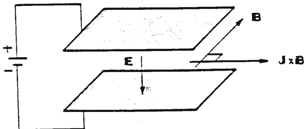
Figure 1.3. Principle of the plasma rocket engine
