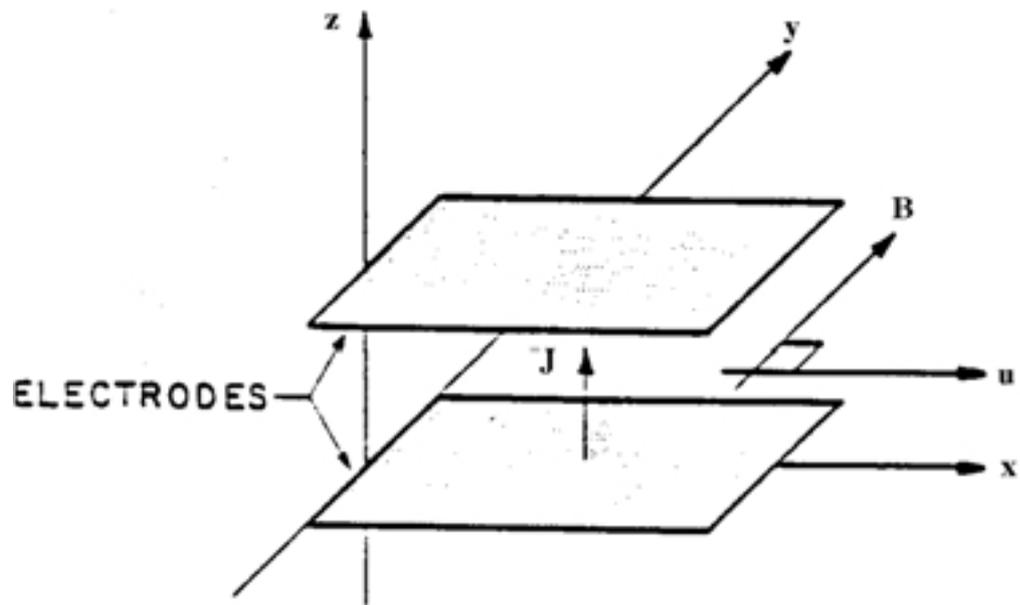
Figure 1.2. Principle of the magnetohydrodynamic generator
